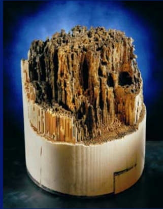
Spectacular Filter Damage Ring-off-Cracks and Melting of the Cordierite Material source Johnson Matthey
