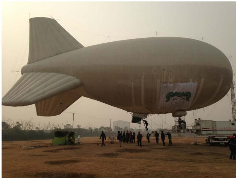
Photo: Balloon used by Shanghai's Environmental Monitoring Center to collect air quality data from an elevation of up to 1000 meters.
