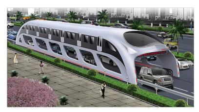
Though it is called the "straddling bus." Huashi's invention resembles a train in many respects — but it requires neither elevated tracks nor extensive tunneling. Its passenger compartment spans the width of two traffic lanes and sits high above the road surface, on a pair of fencelike stilts that leave the road clear for ordinary cars to pass underneath. It runs along a fixed route.
