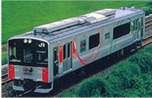
The new train has a diesel engine, two electric motors underneath each car and lithium ion batteries on the roof. The train runs on its batteries until it encounters a hill or the batteries begin to run out and then the diesel engine kicks in.
