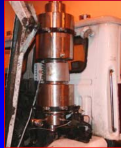
Catalyst-Based Filter with Electric Heater Assist
